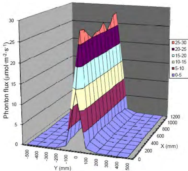
Figure. FR photon flux distribution at the horizontal plane 5 cm below the light source.
