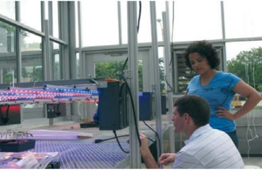
Figure 4. A newly constructed ORBITEC light tower to provide intra-canopy lighting of tall greenhouse crops in two directions within rows. Two-foot-long panels of red and blue LEDs can be switched on or off individually.
