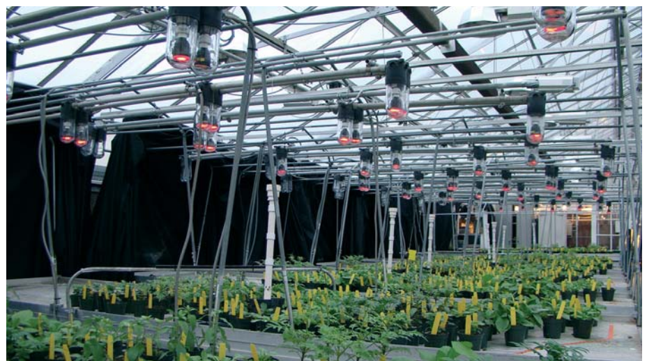
Figure 9. Bedding plant species receive different red: far-red ratios from CCS experimental LEDs during night-interruption studies of floral induction and development being conducted at Michigan State University.
